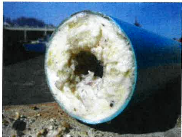
A pipe clogged with thick fats, oil and grease, also known as FOG.
